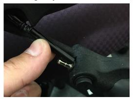
5. Push the air hose onto pump assembly fitting, squeezing the air hose to assist with installation.
