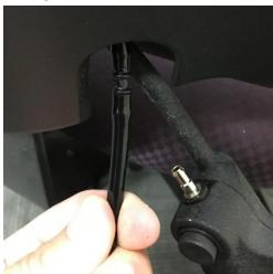
4. Install hose to pump housing. Align the hose to the fitting and cut excess hose so that the air hose will just hit the pump housing when the back height adjustment lever is in the locked position.
