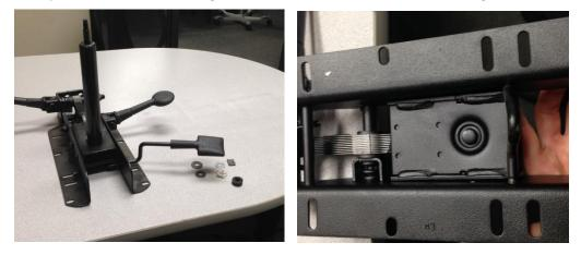
2. Remove the gas lift cannister from the base: Flip the base upside down and hit the cannister with a rubber mallot multiple times until it dislodges from the base.
