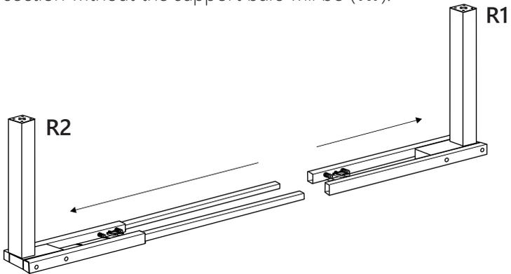
**Step 6:** Insert end brackets (**M**) into the ends of both frame sections, (**R1**) and (**R2**), and fasten each in place with 2x socket screws (**F**). Tighten preinstalled socket screws.
