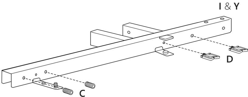
**Step 2:** Attach center leg frame brackets (I) and (Y) to center leg (Q) using 2x socket screws (F).
