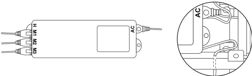
**Step 11:** Plug handset (L) into H port on control box, then run handset cable under frame through inlet hole and place in desired location along any edge.
