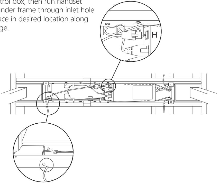
**Step 12:** Make sure no wires are pinched between the frame and work surface, then attach frame to work surface using 24x wood screws (B) into pilot holes.
