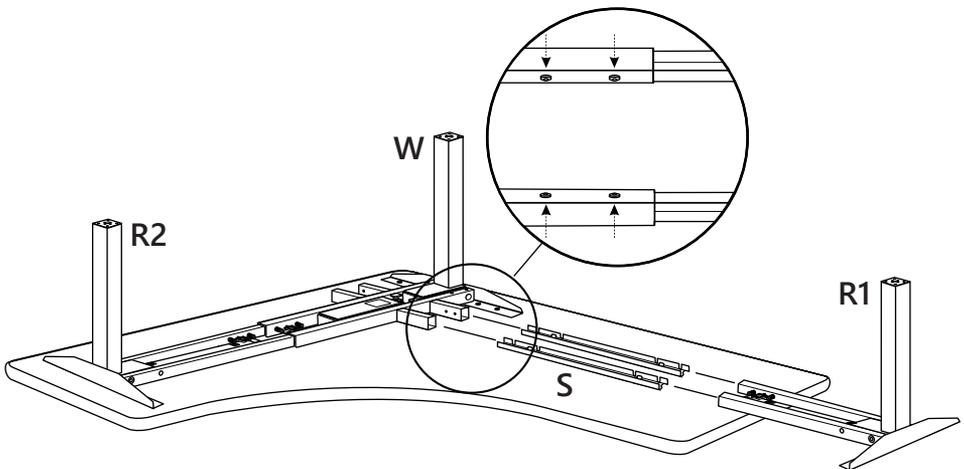
**Step 9:** Adjust entire frame so that the 3x end brackets (**M**) are all aligned with the pilot holes, then lock inner support bars in place by tightening all set screws (**C**).
