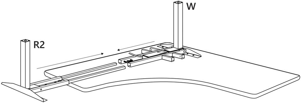
**Note:** If B dimension is less than 55", skip **Step 8** and discard inner support bars (**S**).
