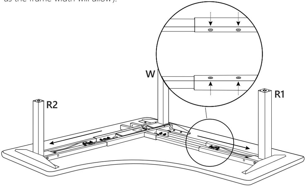
**Step 10:** Run cords from all 3 legs to the center of the frame and plug into ports **M1**, **M2** and **M3**. Run the wire coming from (**R1**) under the frame, through small inlet hole. (**R1**) cable may not be long enough to reach the control box. If this is the case, use leg extension cable (**Z**).
