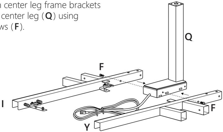
**Step 3:** Insert end bracket (M) into ends of center leg frame brackets and fasten in place with 2x socket screws (F).
