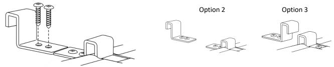
Note: The brackets can be attached farther apart (Option 2) or closer together (Option 3) depending on space requirements on the underside of the work surface.
