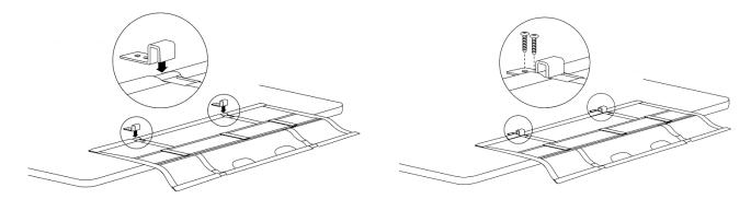
**Step 2:** Place your Open Brackets **(D)** on the work surface in line with the Fixed/Closed Brackets. Fasten the brackets to the work surface using Wood Screws **(B)**.
